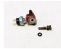
Engine Bleed Valve Replacement
