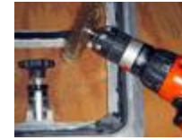
Lexan replacement in the Hatch
